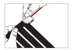
Similarly, also insulate the cuts in the end of the string, as shown in the photo, to prevent oxidation of the braid on the upright at the cut point.
